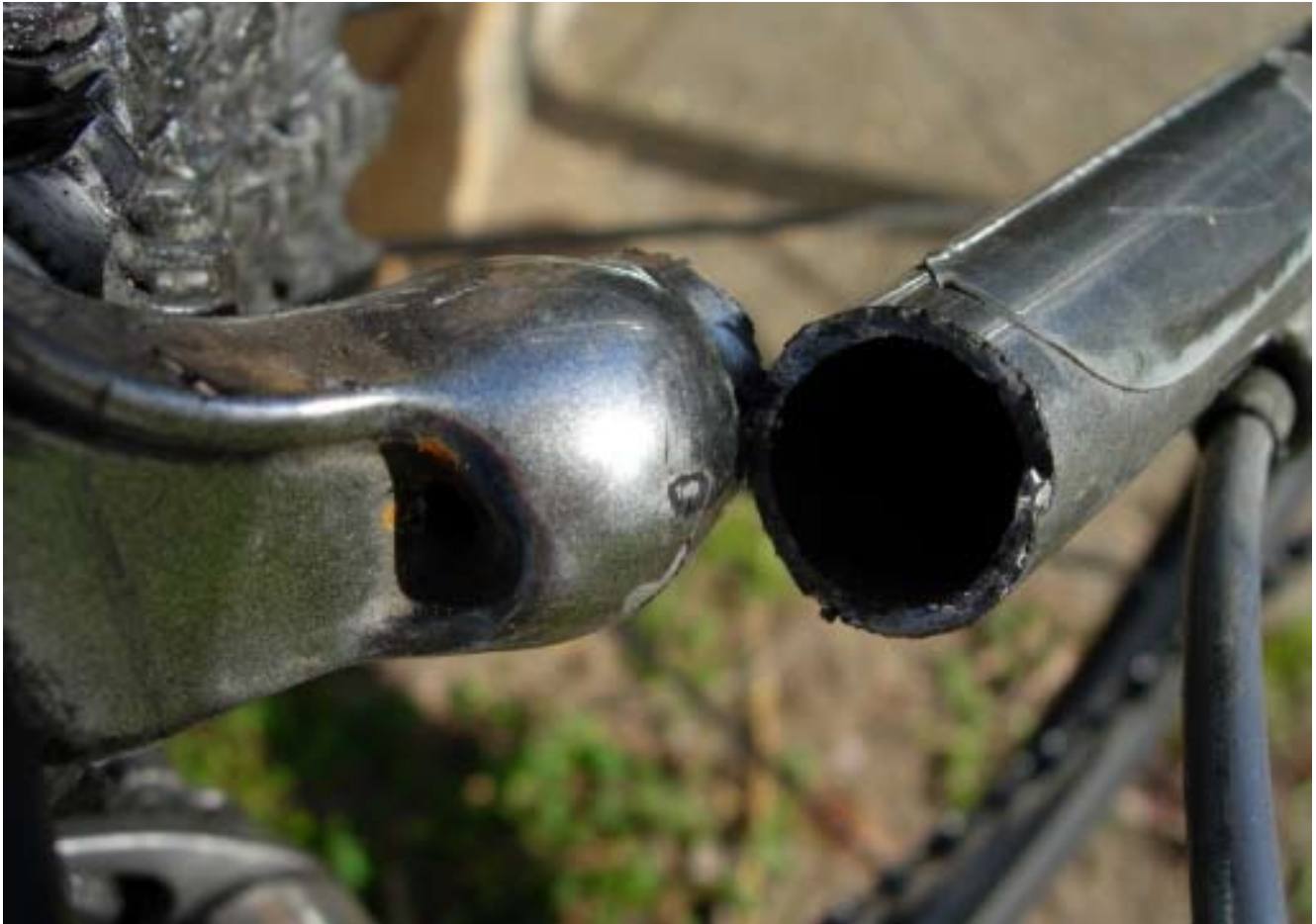
Problem: Clear break of the rear stay.
